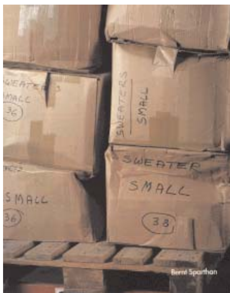
Collapse of boxes under moist conditions
