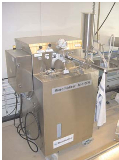
Facility for the manufacture of kilogram quantities of cellulose nanoelements
