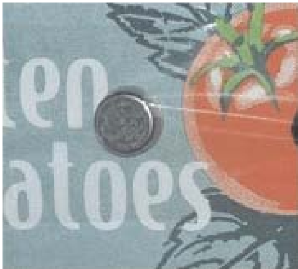
A temperature and relative humidity sensor monitors the conditions in the distribution chain of tomatoes.
